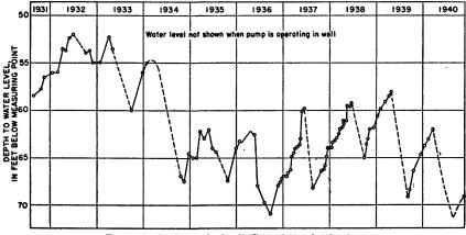
FIGURE 8.--Hydrograph of well (C-35-11) 33aacl, 1931-40.
