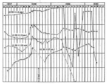
FIGURE 9.-Hydrographs of four wells near the eastern margin of the Coal Creek alluvial fan.
