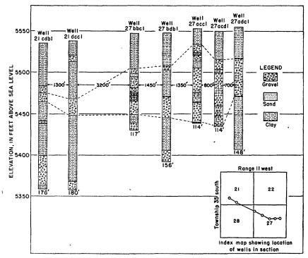
FIGURE 2.-Logs of seven wells in Cedar City Valley and suggested correlations of the coarser sediments.
