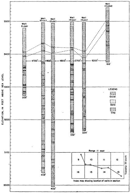
FIGURE 3.-Logs of six wells in Cedar City Valley and suggested correlations of the coarser sediments.
