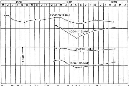
FIGURE 12.—Hydrographs of four shallow wells near Rush Lake showing effects of evaporation and transpiration.
