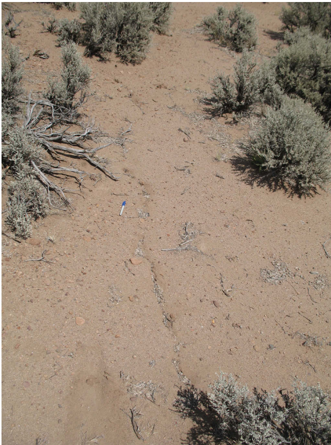
Figure 43. Fissure QWF1 expressed as an uneroded primary ground crack. This fissure could be traced for 900 feet before becoming obscured by recent agricultural activity. Photo taken in August 2009.
