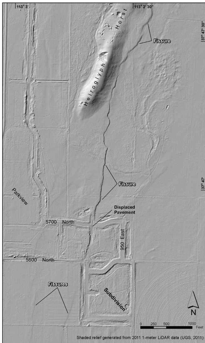
Figure 47. UGS (2011) bare-earth LiDAR image of the south end of the Enoch-graben-west fissures. These fissures exhibit vertical down-to-the-east displacement and are well expressed on LiDAR imagery.
